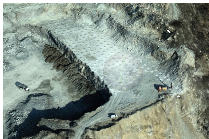
Fig. 4. Drilled blast block imaged by unmanned aerial vehicle (UAV), with a zone highlighted as prospective for differentiated blasting parameters
