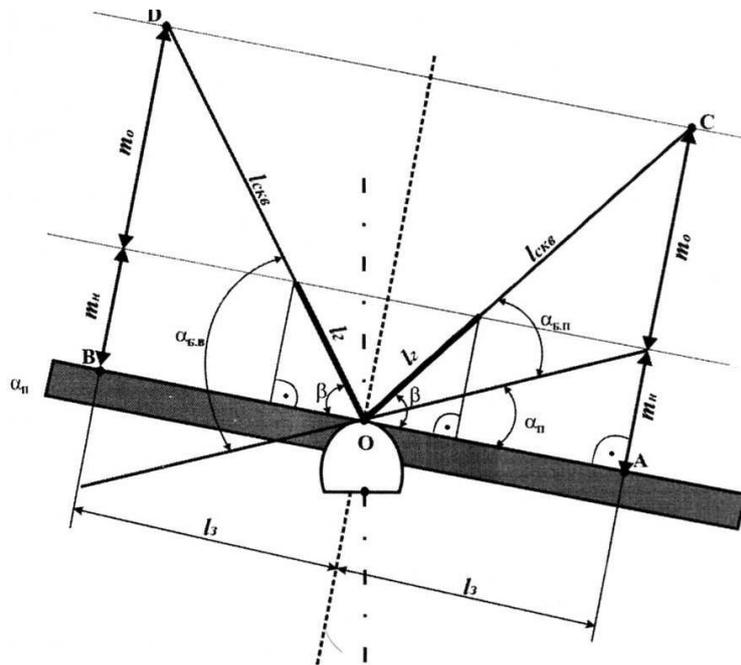
Fig. 5. Calculation pattern for degassing borehole parameter determination
