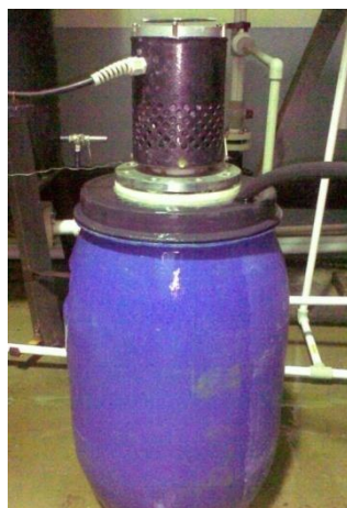
Fig. 5. Installation for the study of hard ultrasound on the ion exchanger grain mechanical strength
