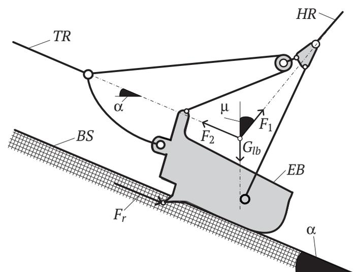
**Fig. 1.** Diagram of forces applied to the bucket: HR – hoist cables; TR – drag cables; BS – face surface; EB – excavator bucket;  $F_r$  – digging resistance forces;  $F_1$  – tension of hoist cables;  $F_2$  – tension of drag cables;  $G_{lb}$  – weight of loaded bucket;  $\alpha$  – angle of face slope;  $\mu$  – deviation of drag cables from vertical direction
