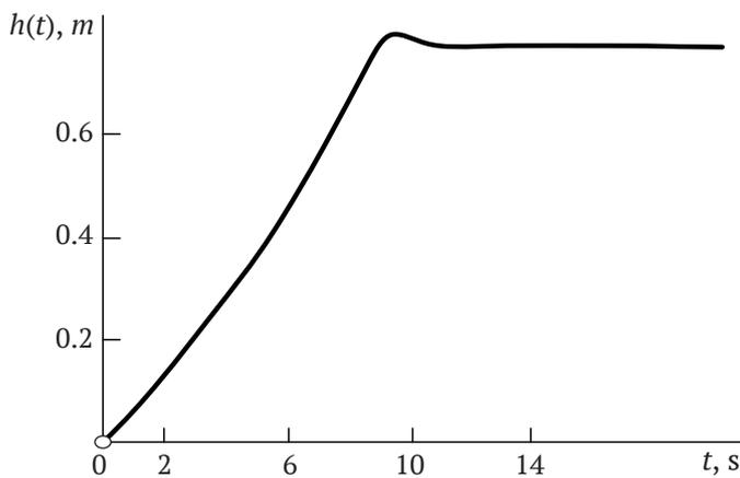
Fig. 9. Depth of cut changes with integral controller
