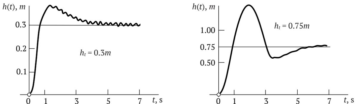
Fig. 8. Changing of cut depth at different parameters of three term controller (PID)
