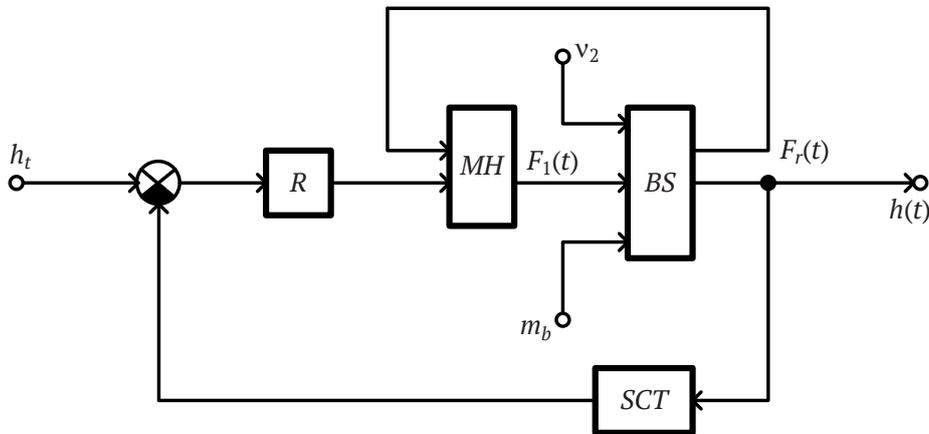
Fig. 7. Digging automatic control system structure:
