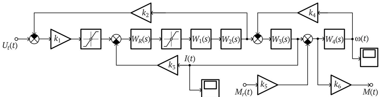
Fig. 4. Schematic diagram of electric drives model:
