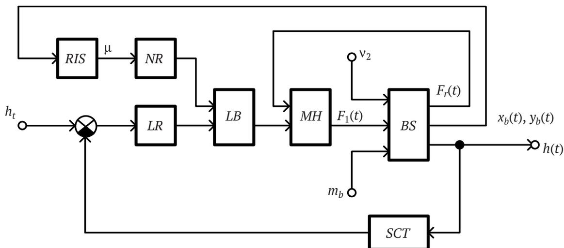
Fig. 11. Structural flowchart of automatic control system of walking dragline digging process: LR – linear controller; NR – non-linear controller; LB – logic block; RIS – hoist cables angle sensor; MH – hoisting mechanism model; BS – face model; SCT – depth of cut sensor;  $h_b$  – assigned depth of cut;  $h(t)$  – current depth of cut;  $x_b(t), y_b(t)$  – current Cartesian coordinates of bucket; block  $F_r(t)$  – current resistance to rock mass cutting
