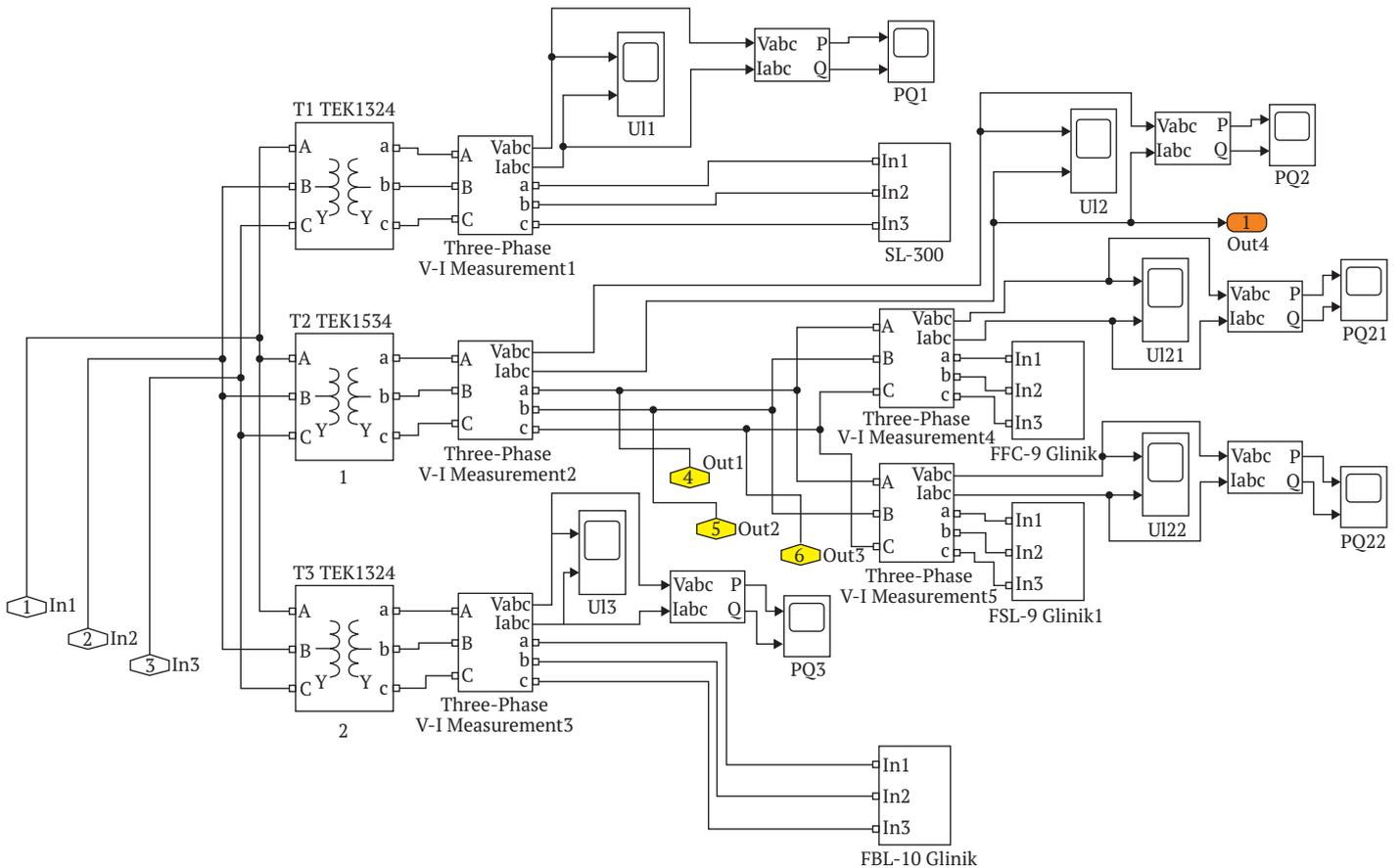
Fig. 7. LOAD (load) subsystem of the simulation model
