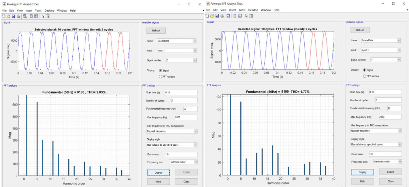
Fig. 9. Results of the simulation modeling of power supply system for a coal mine fully-mechanized longwall with basic process equipment and a resistivity bridge harmonic filter
