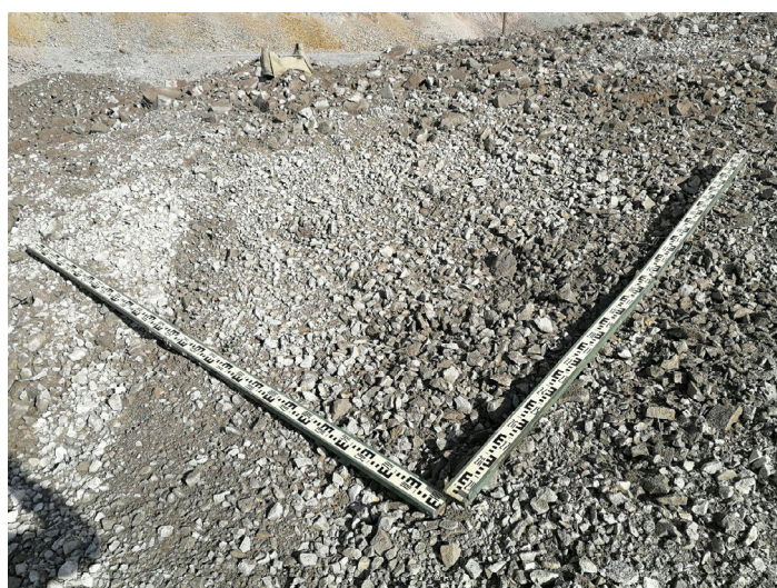
Fig. 11. Results of industrial blasting by means of the developed rock mass fragmentation method
