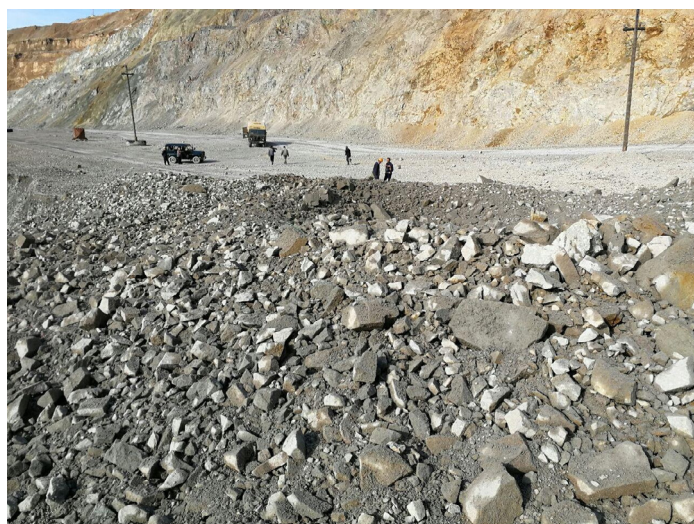
Fig. 10. Results of industrial blasting by means of the traditional rock mass fragmentation method
