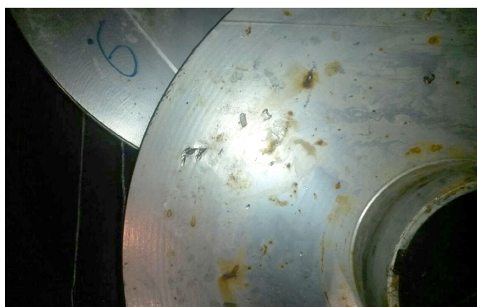
Fig. 5. Adhesion wear of impeller grooves and disks
