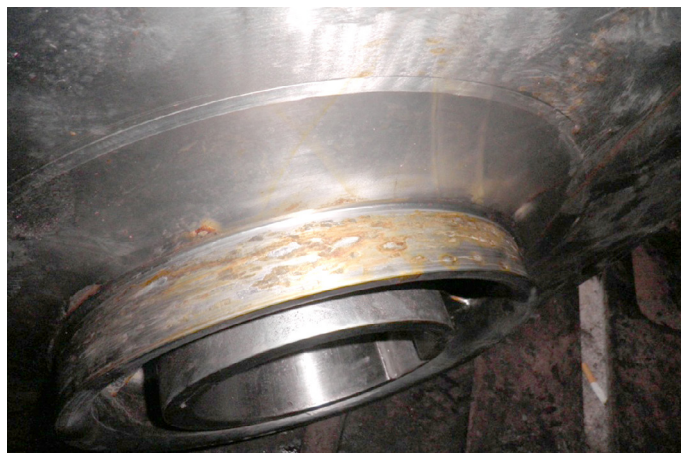
Fig. 4. Corrosion film on the surface of the worn impeller collar
