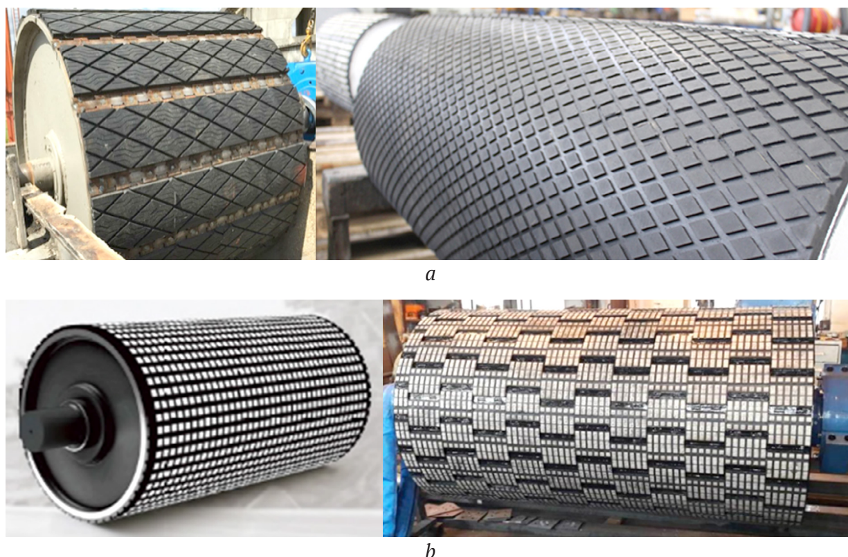
Fig. 2. Types of lining: a – rubber; b – rubber-ceramic
