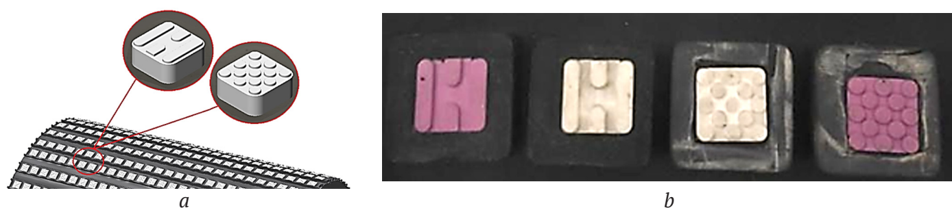
Fig. 8. Digital models ( a ) and prototypes ( b ) of ceramic plates for rubber-ceramic lining
