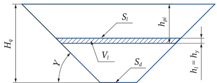
Fig. 3. Scheme for determining the volume of layers to be excavated within a pit envelope:  $S_l$  is layer area,  $m^2$ ;  $S_d$  is bottom area,  $m^2$ ;  $V_l$  is layer volume,  $m^3$ ;  $h_l$  is layer height,  $m$ ;  $h_y$  is bench height,  $m$ ;  $h_{pi}$  height from the top elevation of a pit (daylight surface) to the bottom elevation of a layer,  $m$ ;  $Y$  is overall pit slope angle,  $deg$ ;  $H_q$  is pit wall height
