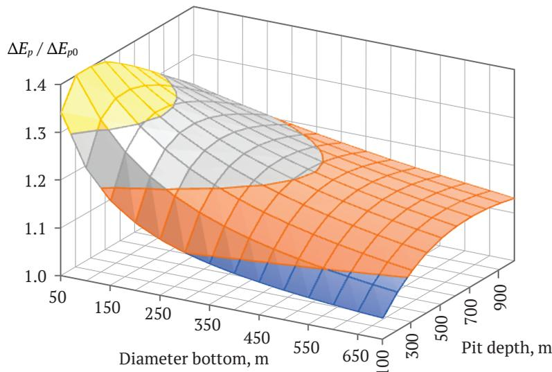
**Fig. 8.** The ratio of energy intensities  $\Delta E_p / \Delta E_{p0}$  depending on the pit depth and diameter of its bottom for the option of the basic pit with an average slope angle of 45°
