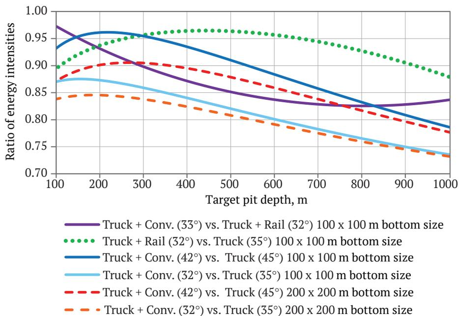
**Fig. 9.** The ratio of total energy intensities ( $Q$ ) of hauling rock mass to the surface from a pit, taking into account the heat of combustion of an initial fuel by mode of transport: Truck + Rail – Dump Trucks + Railway transport; Truck + Conv. – Dump Trucks + Conveyor transport. In parentheses, the average pit slope angle is given
