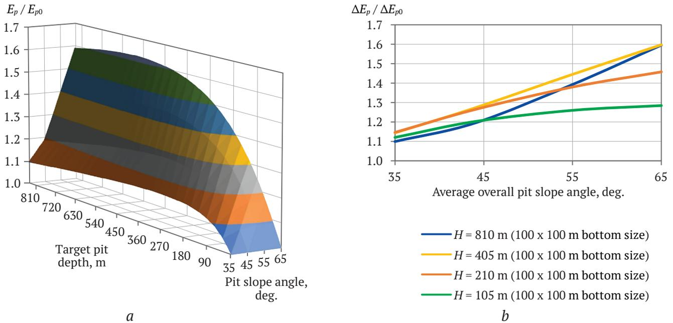
**Fig. 7.** The ratio of energy intensities  $\Delta E_p / \Delta E_{p0}$  depending on the overall slope angle of a basic pit (not taking into account transport berms):
