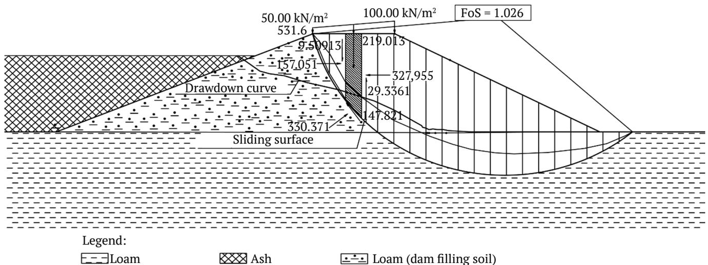
Fig. 5. Computation of outer slope stability for the weakest cross-section through well 324-19 with pipe drainage in place
