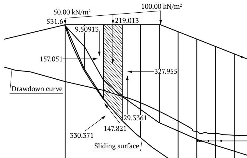
Fig. 4. Computation for cross-section no. 324-19 to identify weaknesses and possible failure points
