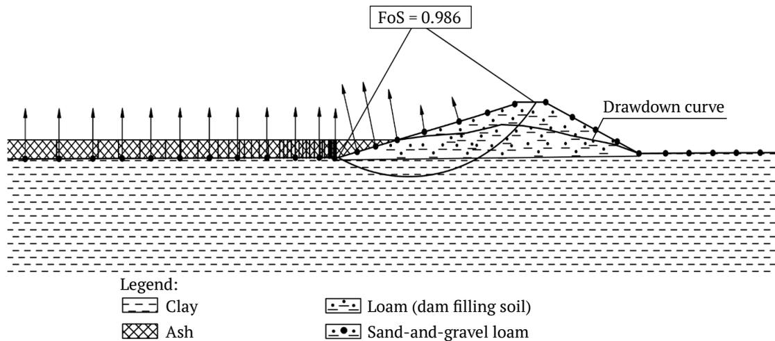
**Fig. 1.** Computations of embankment inner slope stability at characteristic cross-section 324-19 when the dam is watered
