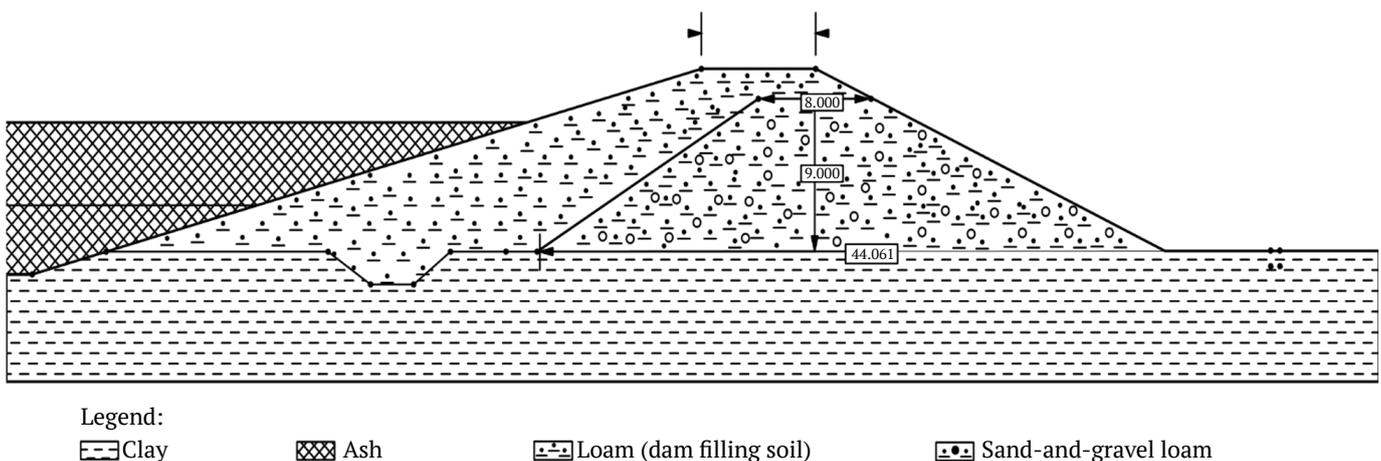
Fig. 6. Structural cross-section of the dam body with cutoff wall and pipe drainage
