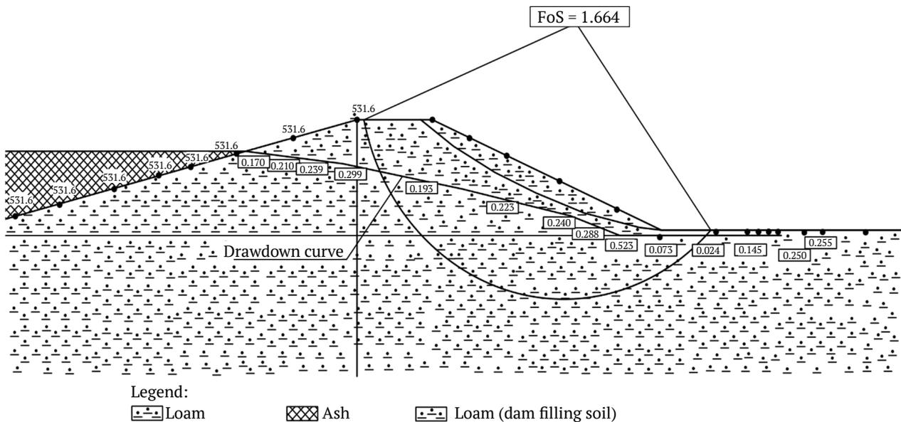
Fig. 3. Drawdown curve and head gradient readings
