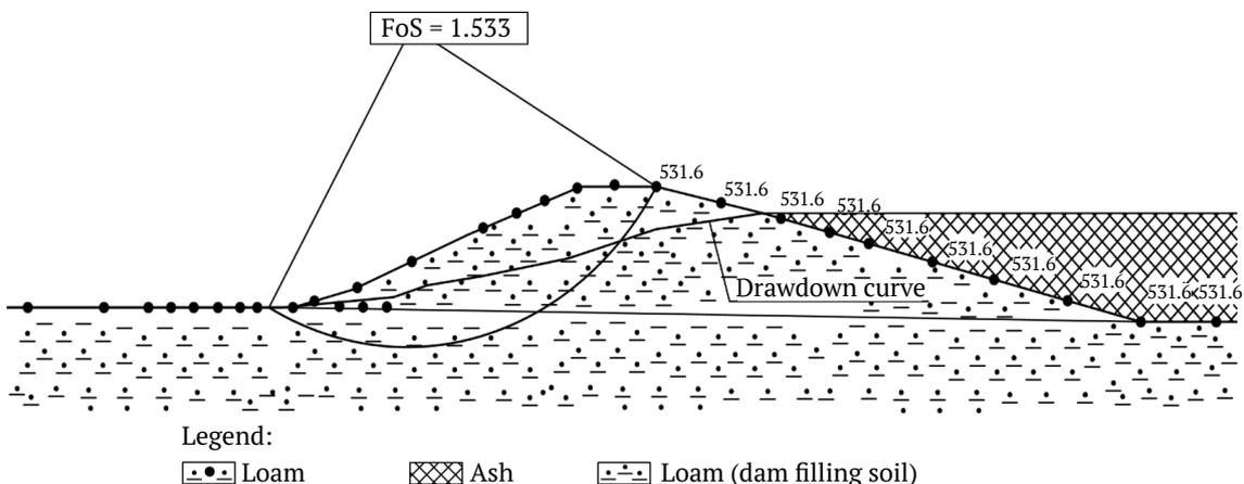
**Fig. 2.** Embankment outer slope stability computations for cross-section 373-19 at a special combination of loads
