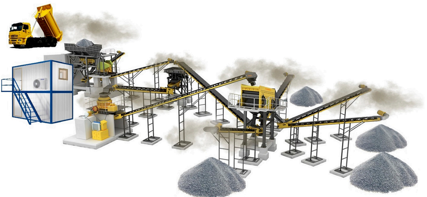
Fig. 2. Schematic of the crushing and screening plant illustrating the main sources of dust generation
