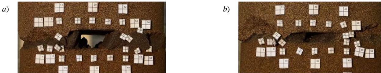
Fig. 6. Seam EM deformation schematic – rock mass with a mine working junction
