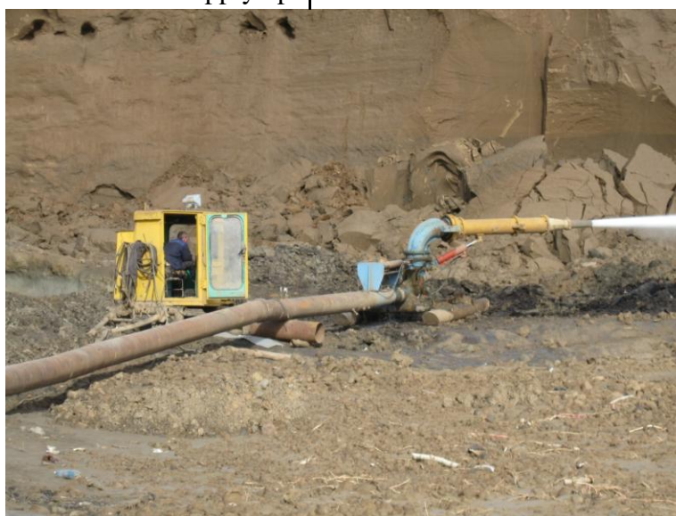
Fig. 1. GD-300 hydromonitor made by Zavod Gidromash OJSC at Kedrovsky mine.
