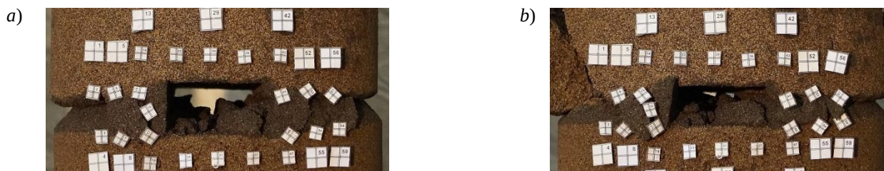
Fig. 5. Seam EM deformation schematic – rock mass including a single mine working
