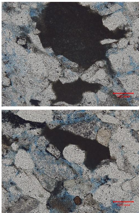
Fig. 15. Pore space filling with carbonate material based on thin section photographs in transmitted light
