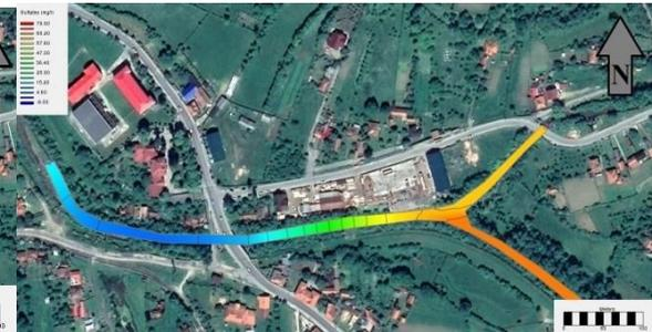
Fig. 11: Concentration of sulphate in 2 hours
