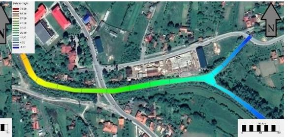
Fig. 13: Concentration of sulphate in 8 hours
