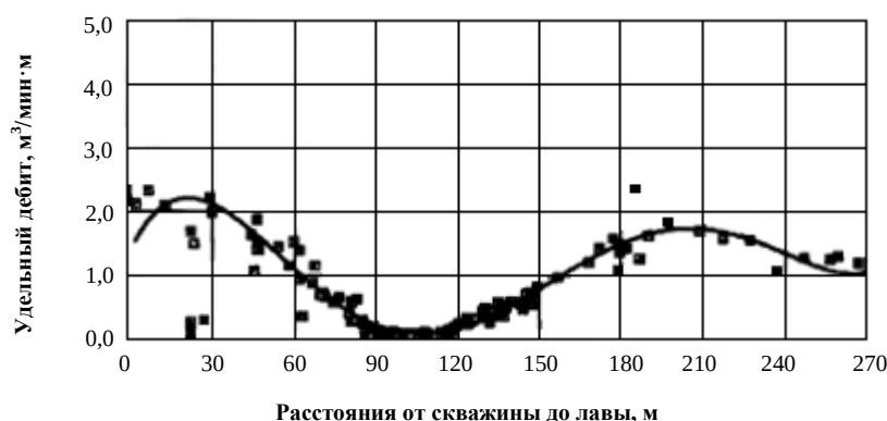
Fig. 2. Change in degassing borehole flow rate at Picket53+1 m after HDA
