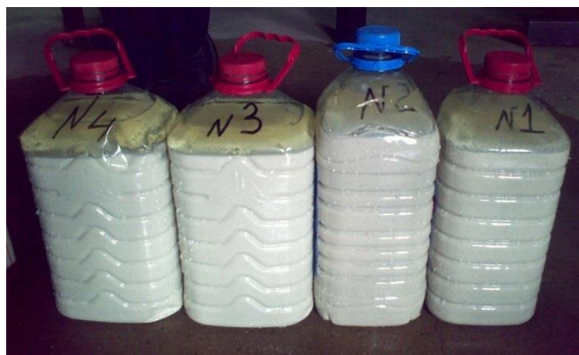
Fig. 6. Samples of the initial new ion exchanger (Nos. 3 and 4) in comparison with the samples of the previously used ion exchanger (Nos. 1 and 2)
