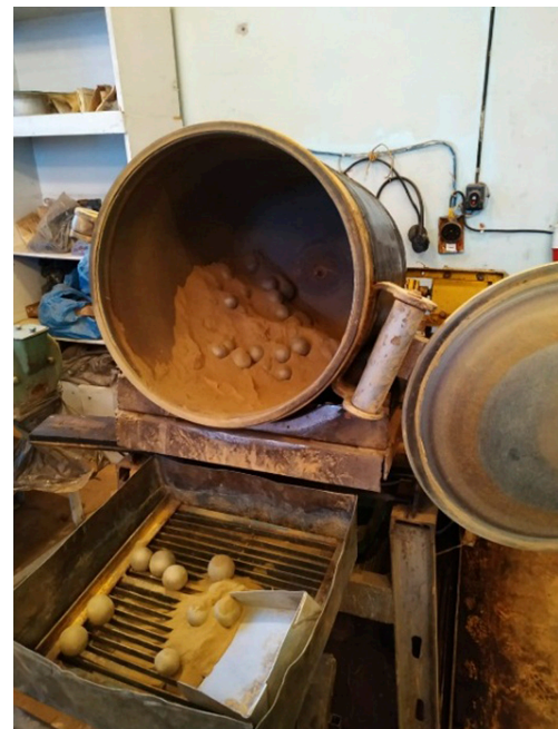
Fig. 2. Laboratory MSHL-120 ball mill
