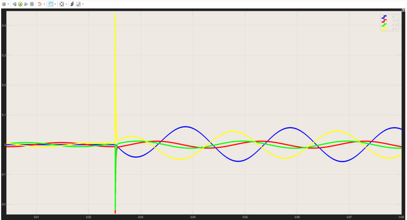
Fig. 5. Oscilloscope pattern of the leakage currents through insulation, human body, and RCD tester circuit with an RC filter
