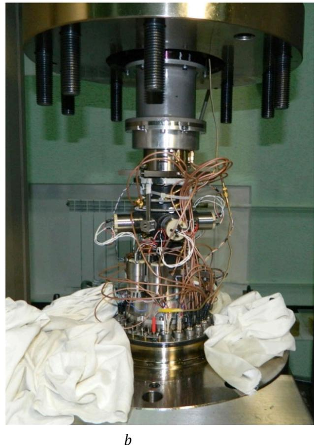
**Fig. 5.** Basic diagram of the experiment (*a*) and sample prepared for tests in the triaxial compression chamber (*b*) with installed acoustic emission sensors:
