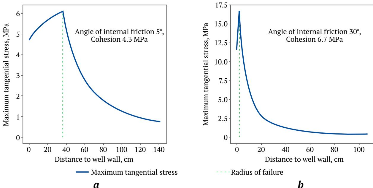
**Fig. 7.** Distribution of maximum tangential stresses in the vicinity of open-hole well for the following parameters: Poisson's ratio – 0.25; overburden rock stress – 26.06 MPa; initial pore pressure – 11.0 MPa; depression – 10 MPa; wellbore radius – 0.1 m
