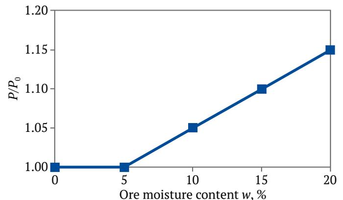
Fig. 4. Dependence of the  $P/P_0$  ratio on the moisture content  $w$  of the spilled ore
