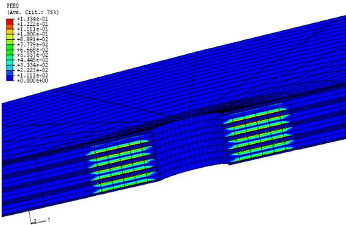
**Fig. 8.** Numerical solution of the problem of stress distribution in the vicinity of perforation channels at a perforation density of 8 perforation holes per 0.3 m for a cased well. The blue color indicates the elastic zone, while other colors indicate the zone where the shear failure criterion is met [15]
