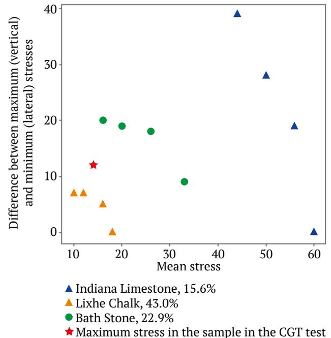
Fig. 6. Compaction failure envelopes according to [8] and ultimate stress state for a Tournaisian stage rock sample
