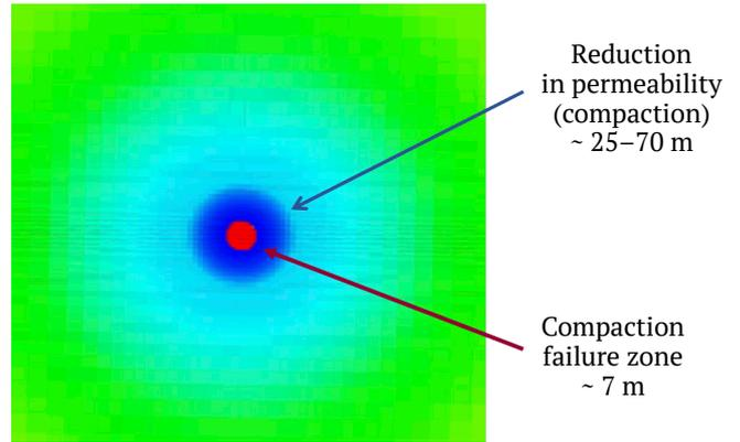
**Fig. 10.** Permeability multiplier distribution based on the computations using a coupled model in tNavigator (hydrodynamics + geomechanics) with a script to account for compaction and compaction failure through effective stress analysis. The colors are explained in the text
