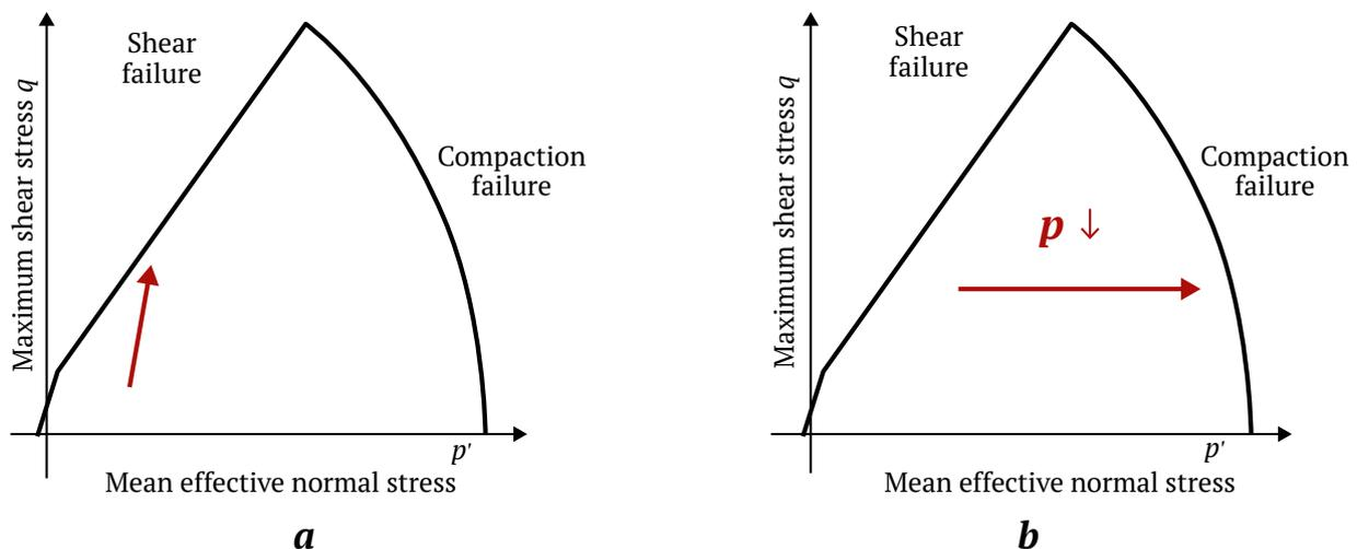
**Fig. 3.** Failure diagrams and direction of change in effective stresses in experiments simulating the effective stress field in the vicinity of a vertical open hole well (a) and in experiments with changing pore pressure (b)
